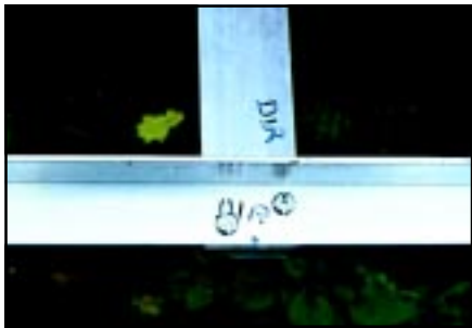
An angle section bolted to the boom.
